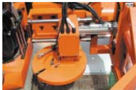
The 8 position Automatic Tool Changer with protective dust cover
