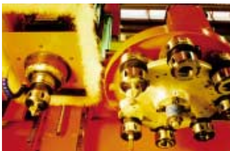
The SELEXX series provides the proven and reliable ANDI spindle, with HSK 63 F tool holder and 8 position carousel tool changer - standard on all SELEXX models.
